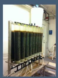
Sintef column system including a water reservoir
